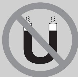
The encoder wheel must be protected against strong magnetic fields. Otherwise, the encoder wheel may be damaged.
