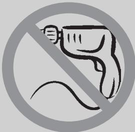
The hub retaining nuts must be fitted and tightened by hand. An impact wrench must not be used under any circumstances to install the brake disc or attach the hub retaining nut.
